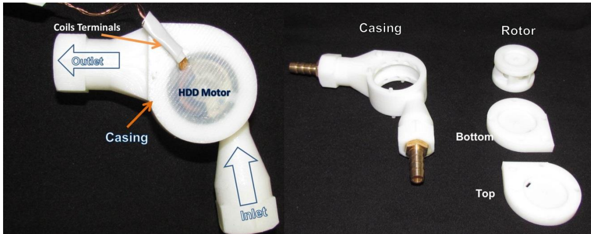
Figure 4.5 Notched model, scale 3.175X, 2.5 inch HDD motor.
